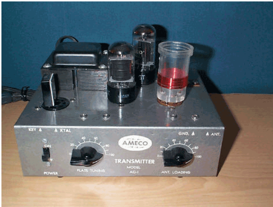
Ameco AC-1 Transmitter – plug in Crystal at left
