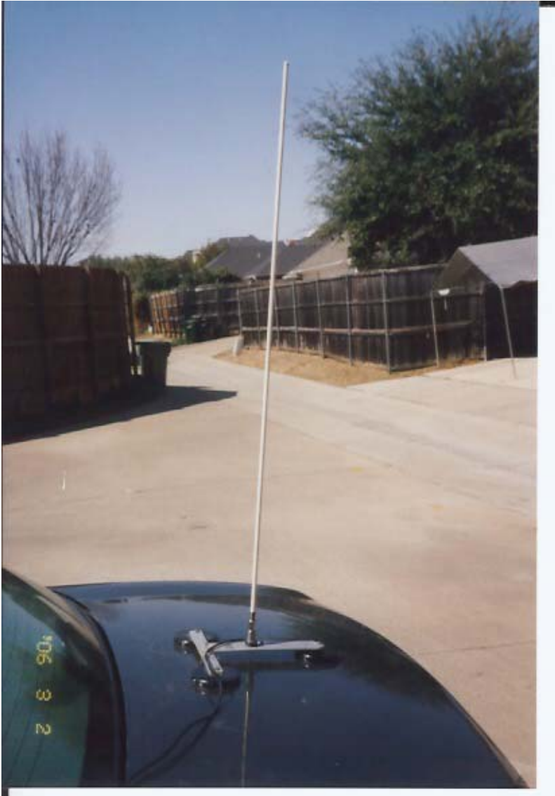
Prototype Nanotube Antenna, 34 inch long \frac{1}{4} wave 27 Mhz antenna
