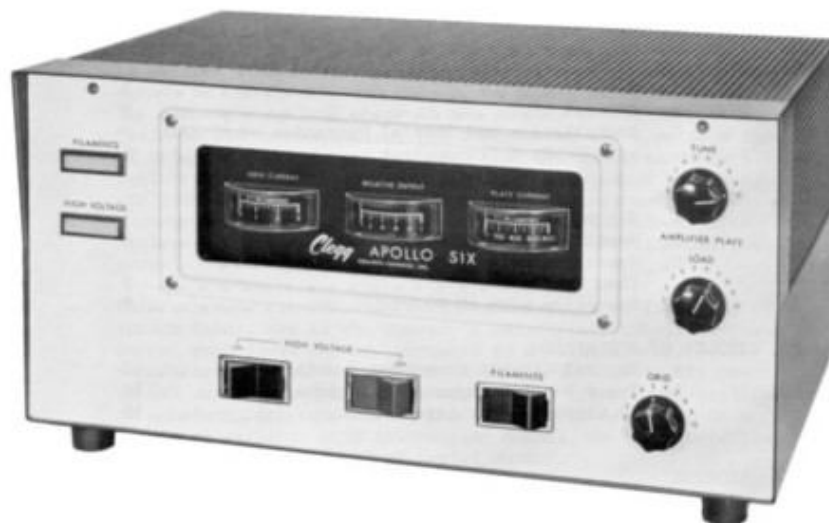
Clegg Apollo Six Meter Linear Amp 15w in 375w out
