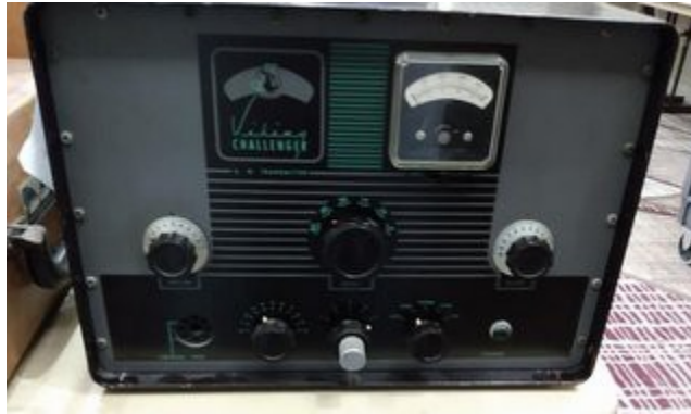
Johnson Viking Challenger Transmitter $85 70W AM/120W CW Internal Power Supply Needed external VFO otherwise xtals
