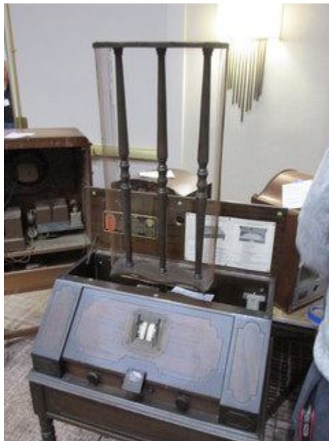
Radiola with rare AG-814 Loop Antenna
