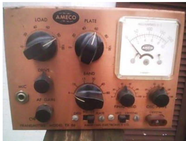
Ameco TX – 86 80-10 transmitter
