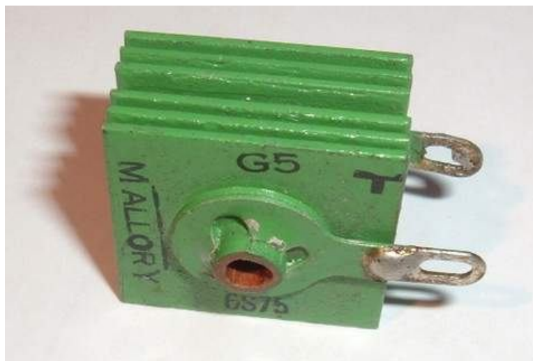
Typical Selenium Rectifier for 121VAC
