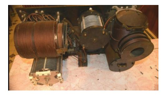
This is just the 'tuner' part of the receiving setup. You'd need a separate detector, which could be a crystal (catwhisker type) or primitive tube detector. It's long wave – like 30 KHz to 300 KHz.
