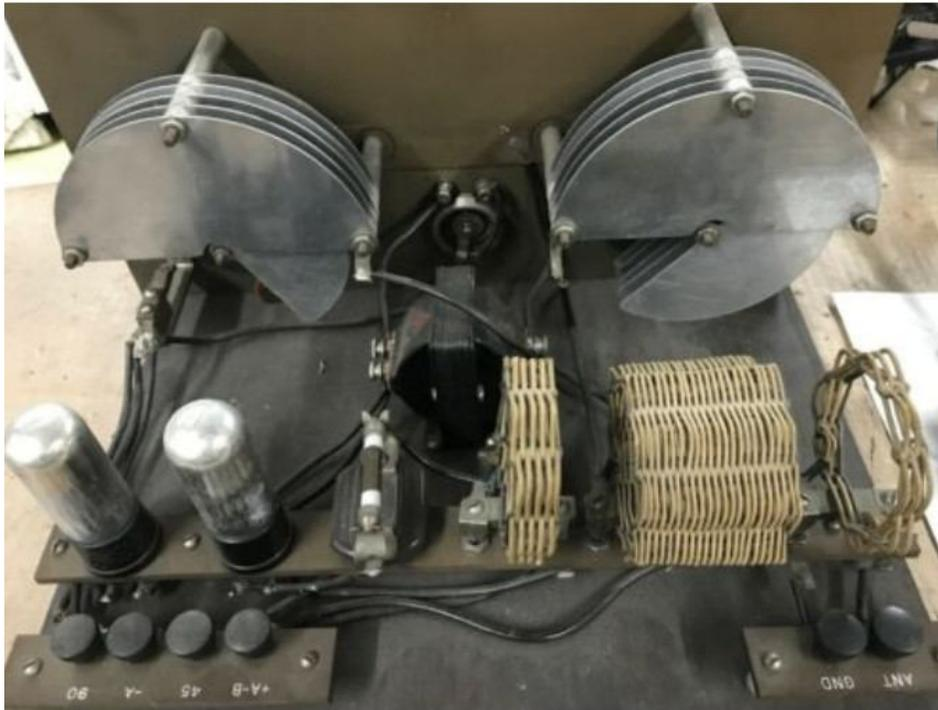
This kit uses a pair of '99 tubes – one regen detector, one audio stage. This is one of the very first 'shortwave radios'. The UV-199 triode tube was made for “portable radios” and takes 3v at 60 ma. It had a unique base not used by any other tube! Most of the home radios used the UV-201 tube that took 5-6v at 250 ma. However, with a smaller filament, life was usually much shorter due to vibration killing the tube. It was fairly fragile. It fell out of use after 1926.
