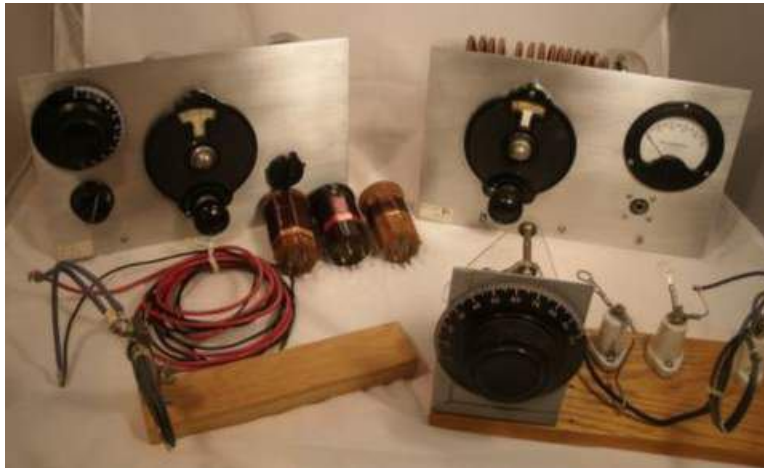
Regen RX, Hartley TX Coils for 160/80/40m – plug in Ant tuner is front right
