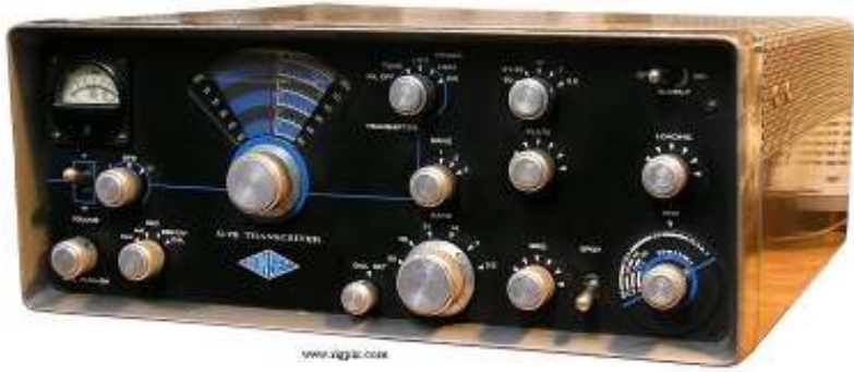
Gonset G-76 Transceiver AM/CW no SSB Needless to say, without an SSB rig, Gonset faded from the HF scene.
