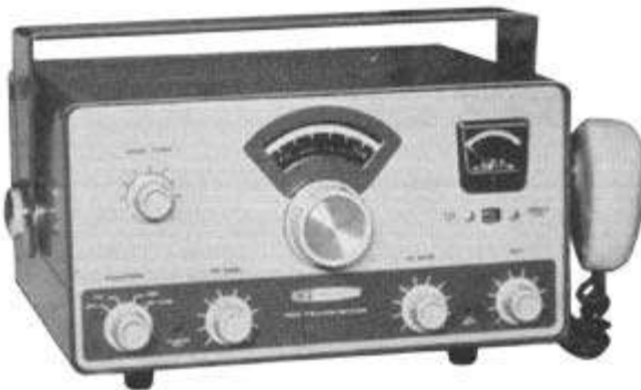
The HW-12 (75m), HW-22 (40M) and HW-32 (20M) Transceivers
