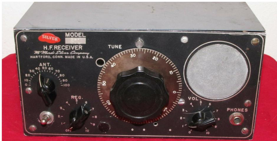
There were two versions of this. One used 1.5v tubes – for battery operation. The other used 6v tubes for operation of a separate power supply off the a/c line.
