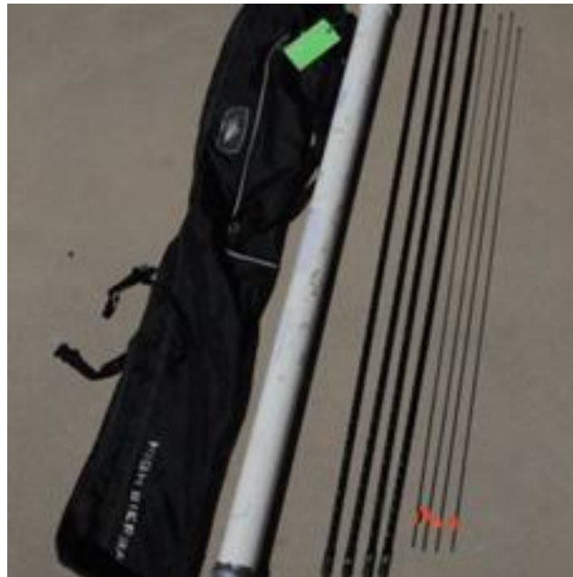
Hamstick Antennas in PVC pipe carrier
