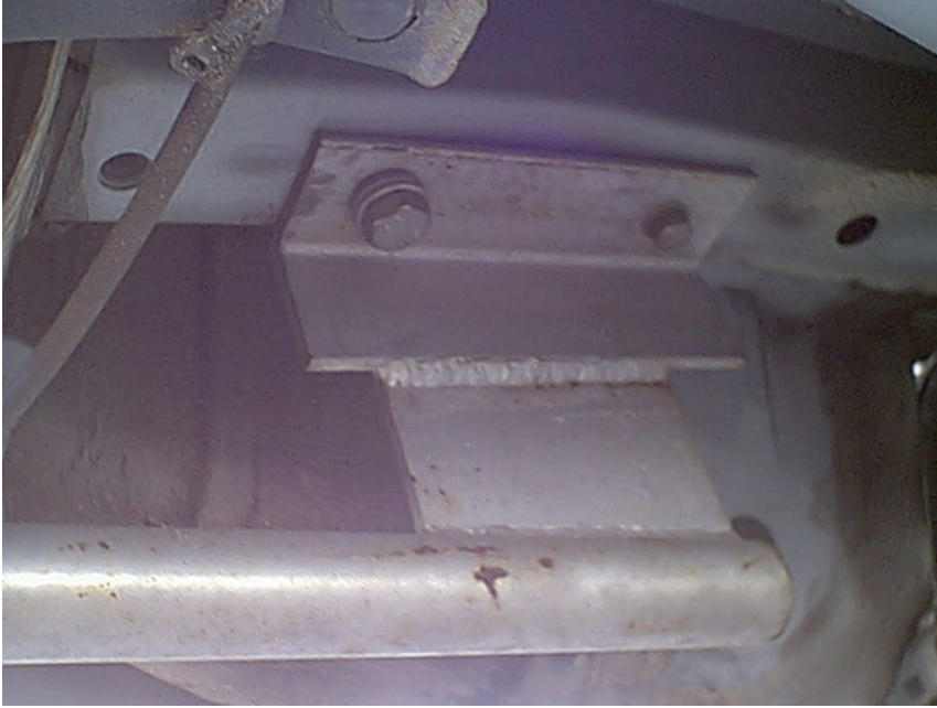
Bracket underneath using 'tow hook' holes
