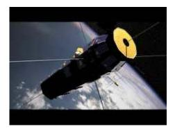
CINDI and C/NOFS were designed to study disturbances in Earth's ionosphere that can result in a disruption of navigation and communication signals. The ionosphere is a gaseous envelope of electrically charged particles that surrounds our planet and it is important because Radar, radio waves, and global positioning system signals can be disrupted by ionospheric disturbances.
