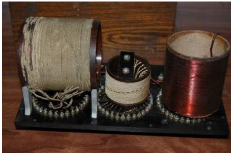
General Electric Type D crystal set insides
