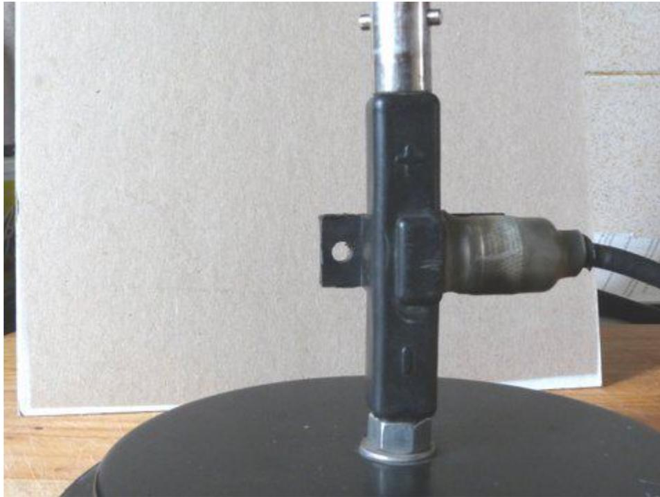
I then sealed the PL259 with impregnated heat shrink and it has worked perfectly for about 4 years.
