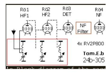
You could switch in a narrower audio bandpass filter for CW. The set had 3 tuned circuits giving fairly decent selectivity – sensitivity was about 10 microvolts on both AM and CW. It was stable enough to tune in SSB transmissions (which didn't occur back then).
