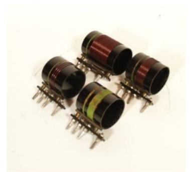
Plug in Coils for Model CS-5
