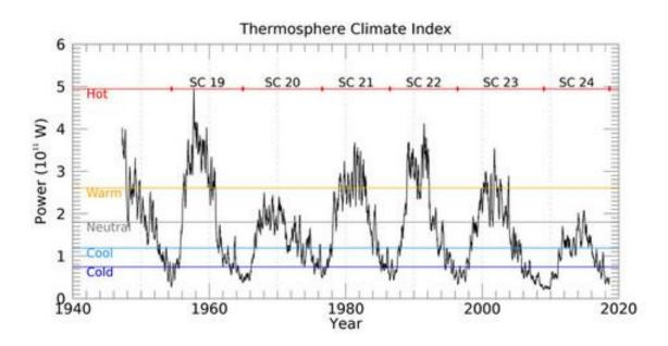
These results come from the SABER instrument onboard NASA's TIMED satellite. SABER monitors infrared emissions from carbon dioxide (CO2) and nitric oxide (NO), two substances that play a key role in the energy balance of air 100 to 300 kilometers above our planet's surface. By measuring the infrared glow of these molecules, SABER can assess the thermal state of gas at the very top of the atmosphere–a layer researchers call "the thermosphere."
