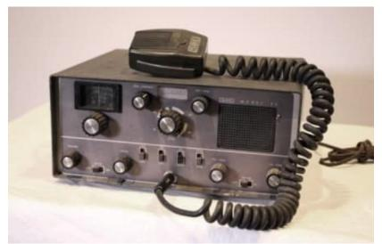
SBE 34 Mobile Transceiver Solid State with 2 tubes in TX
