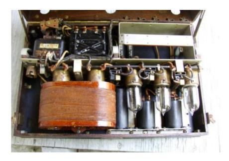
The dimensions of the box were 17 inches by 10 inches by 7 inches and weighed 21 pounds. The A-21 retractable antenna was located in the rear of the aircraft and was expanded by the air observer while in flight. It could reel out to 300 feet in length, was made out of two copper wires and weighed 19.5 pounds. Depending on the amount of antenna allowed behind the airplane, the antenna functioned at a wavelength of 750 kHz
