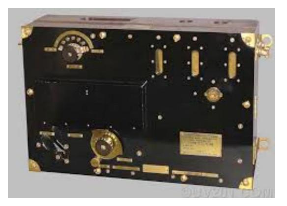
The SCR-68 range was reliable within a five-mile radius, a serious issue when the airplane needed to travel long distances. Another issue with the SCR-68 was the static noise that came from the "ripples" in the generator commutation. The noise was faint and was only considered a problem when receiving messages that exceeded 5 miles
