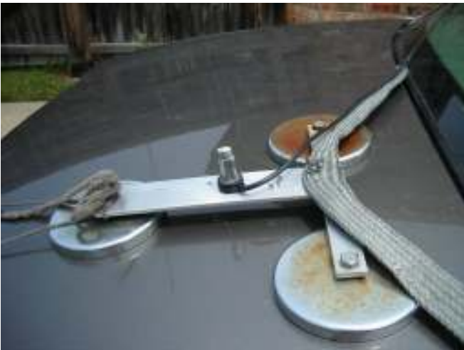
Mag mount with fractured mast
